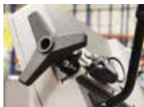
Saw blade break monitoring the saw blade tension is fitted with a saw blade tension monitoring and saw blade break monitoring device
