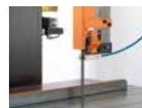
Standard height-adjust- able guide arm
