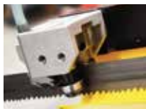
Saw blade guide made from carbide
